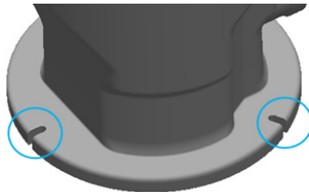
Figure 2 – Floor fixation notches
