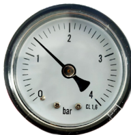
Figure 16 - If the pressure is 0.3 to 0.5 bar higher than the reference pressure Pr: maintenance of the cartridge required
